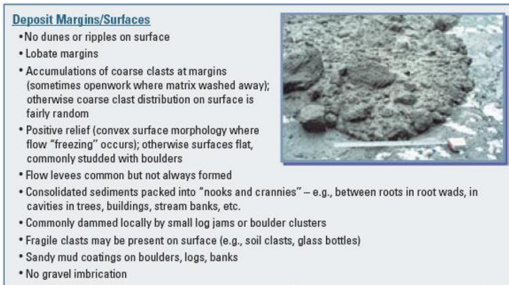
Figure 4.33. Field Evidence of Debris Flow
